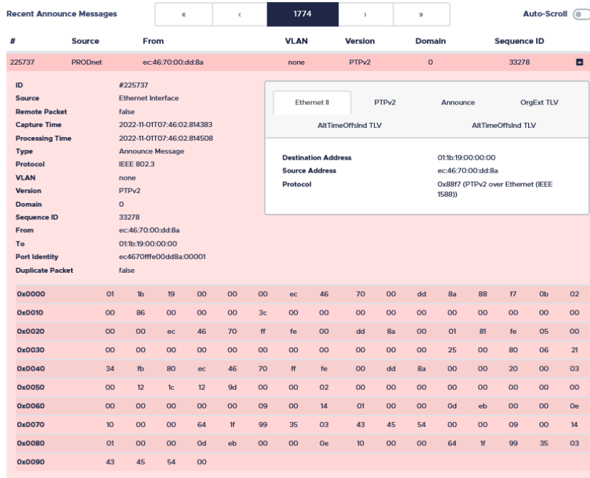
Figure 7.3: Breakdown of a PTP Message
